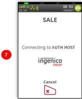
Terminal connects to the acquirer using the configured connection method e.g. 'Mobile Network'.
