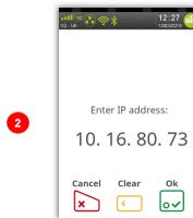
Press to confirm address or clear the digits and re-enter new address.
