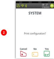
Press button to print 'System Configuration', press to skip or press to exit function.
