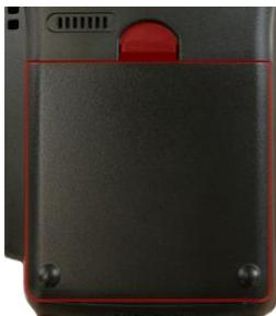
To insert or replace the SIM card in the terminal, turn the axept® S900 terminal over so the battery cover latch is visible.
