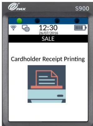
The cardholder receipt will then begin printing and can be torn off once printing has completed and axept® S900 will return to the main menu.
