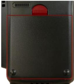
To insert the battery, turn the axept® S900 terminal over so the battery cover latch is visible.
