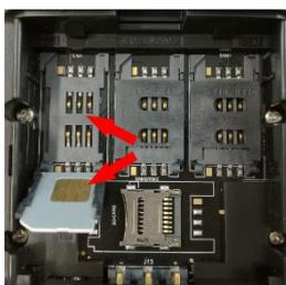
Place the new SIM card in the slot making sure the contacts of the terminal match the contacts of the SIM (the contacts of the sim should be at the base facing away from you) and close the latch.
