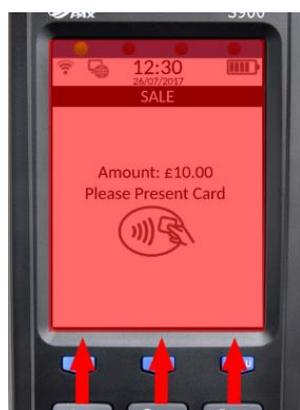
Position the (contactless enabled) card or device around the screen area of the terminal for a few seconds until a 'beep' sound confirms the card has been read (the green contactless LEDs will incrementally light up as the card is being read).
