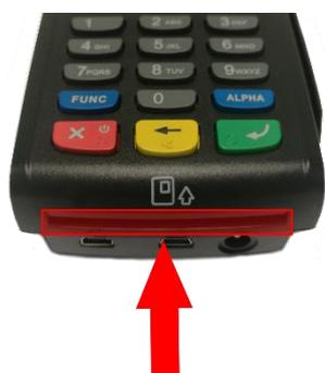
Insert the card (with the Chip of the card on top, facing towards you) into the Chip and PIN card slot at the base of the terminal.
