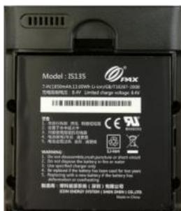
If the battery is already in place, remove the battery from the terminal by gently lifting the battery away from the terminal.
